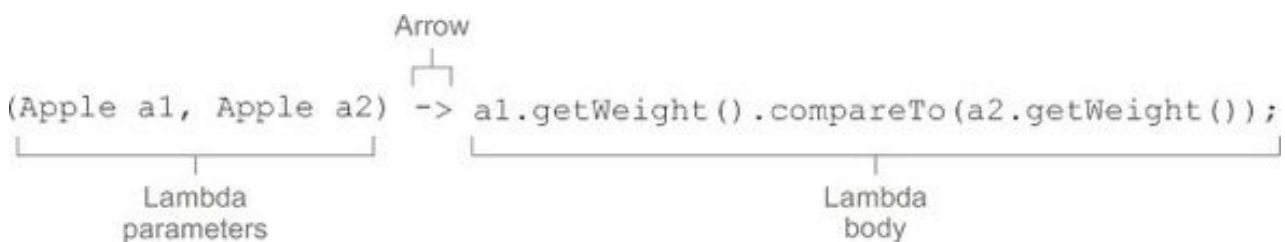
Figure 3.1. A lambda expression is composed of parameters, an arrow, and a body.
